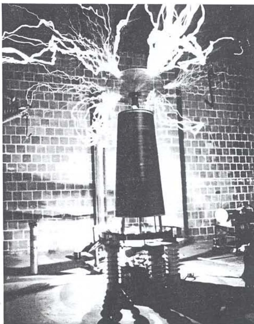
**Figure 6. The Basic Tesla Coil.** The author worked on this Tesla coil constructed by Dale Travois. Tesla coil construction and operation is an excellent way to begin learning about the intricacies of high voltage-high frequency electricity. Photo by Aubrey
