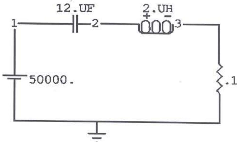
**Figure 1. The Basic Representation of the Internal Dynamics.** During the initial experiments, 2 $\mu$ F were used. During later experiments, the capacitance was increased to 12 $\mu$ F. Connections inside and outside of the capacitors have inductance and resistance.
